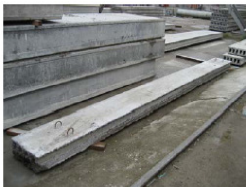
Figure No.6 A narrowed slab with lifting eyes
